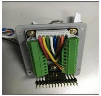
Figure 59: Wiegand Interface Cable
